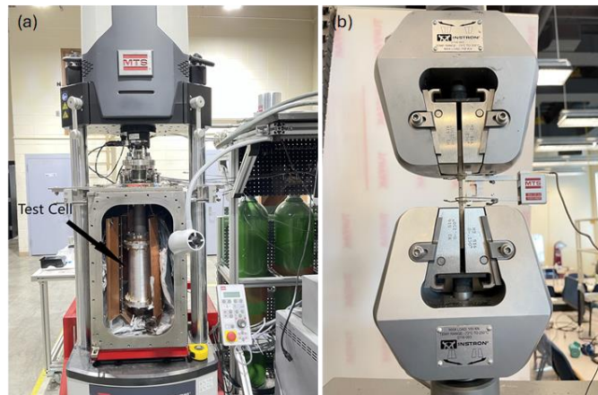
Figure 2. (a) Cryogenic Accelerated Fatigue Tester (CRAFT) setup, and (b) Instron 2716-003 tensile testing machine.
